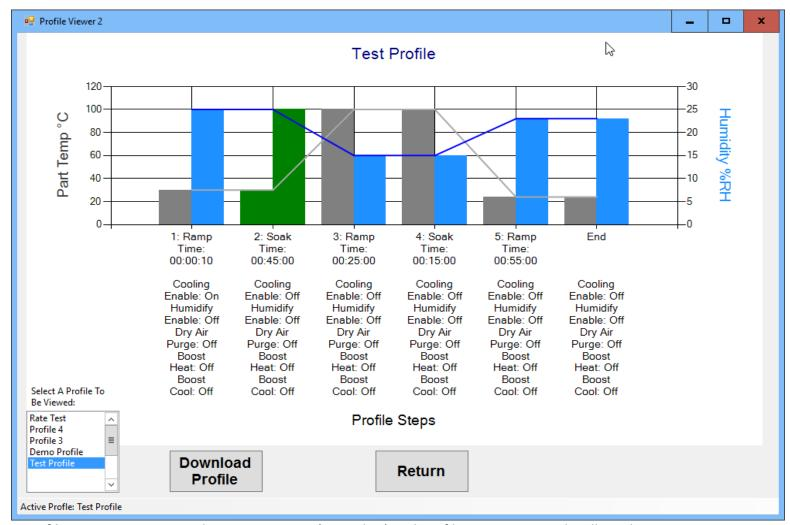
**Profile Viewer Screen:** Displays Current Step (green bar) and Profile Programs Graphically with Output Events.
