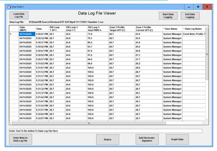
**Real-Time Data Log File Viewer Screen:** Displays data as it is being logged to the PC file for peace of mind and to make sure the correct data is being logged. Events are also recorded in the Data Log file along with Batch Information and Min/Max process values for each input. Notes can be added by the operator real-time as the profile or batch is running. Multiple electronic signatures can be added to data log files for tamper-proof security.
