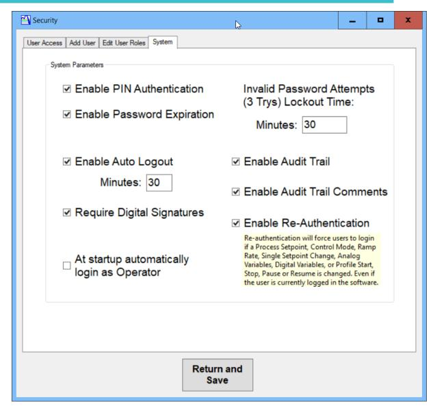
**Security Screen – System:** The Security System tab allows for advanced user management and enables the use of digital signatures and or audit trails.
