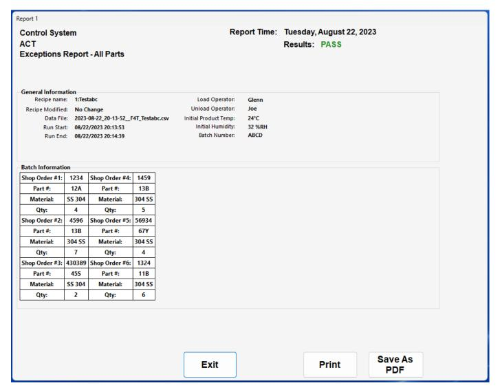
**Quality Assurance Reports:** Customizable Quality Assurance Reports can be automatically generated after a profile run. PASS/FAIL criteria can be based on a uninterrupted profile, alarm condition or a tolerance band setup on a particular step or steps in a profile. User input and automatic fields filled in after the report is generated are customizable to your application.
