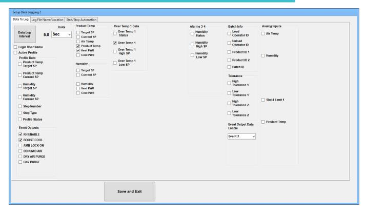
**Data Log Setup Screen**: All Process Data and Profile Status parameters can be logged to a CSV Excel file. Data can be logged as Encrypted if required with a password.
