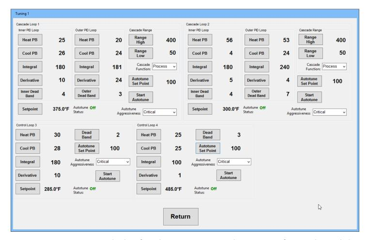
**Tuning Screen:** Easy tuning can be done from the tuning screen. Use the Auto Tuning function along with the real trend graph to finely tune your process!
