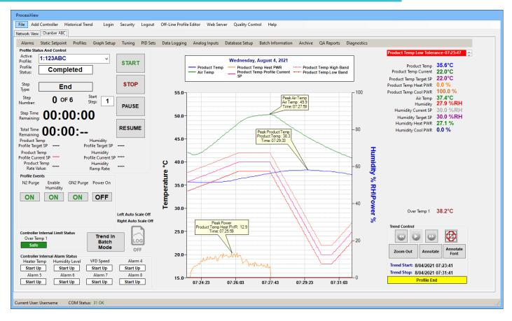
**Dedicated Overview Screen:** Each Controller/Chamber on the network shows real-time trend, process data, event output status and current Profile status. Profiles can be started, stopped, paused or resumed from this screen. Profile Events can be manually turned on or off if enabled.
