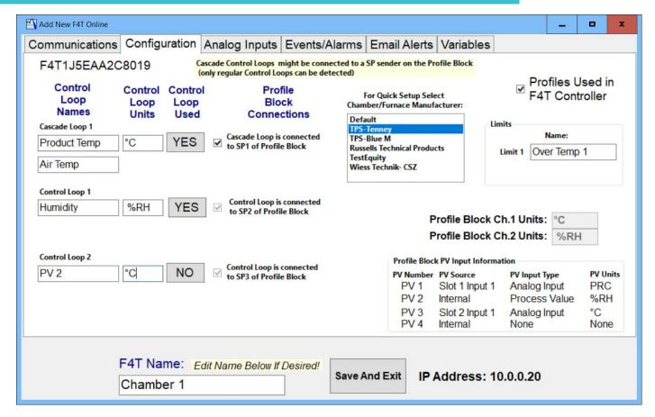
**Setup Screen:** Predefined manufacturers setups are included making setup very easy! Sensor inputs can be given custom names to make the interface more intuitive to the user. (TPS-Tenny shown selected above). No programming required!
