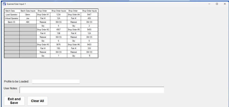
**Code Scanner Setup Screen:** Operator input for batch processing can be entered with bar codes for quality and product accuracy. Profiles can be loaded based on bar code information as well.
