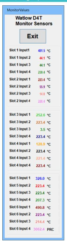
**D4T Monitor Screen:** 24 external sensors that can be data logged and viewed in the software. ProcessView supports an additional Watlow D4T that can be used to add up to 24 external sensors to a chamber or for a device under test.
