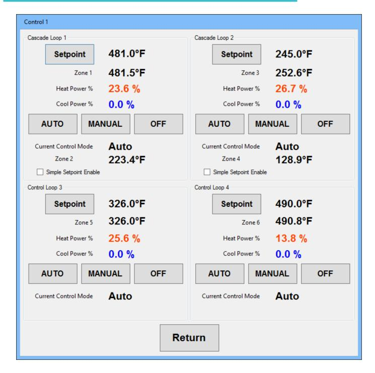
**Static Setpoint Screen:** Control parameters such as control mode (Auto, Manual or Off), Static Setpoints and ramping mode can be adjusted by the user. For Cascade control users can enable Simple Setpoint when not requiring Cascade control usually used for controller to a Part Temperature.
