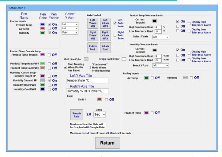
**Graph Setup Screen:** The Graph Setup screen allows the User to choose what paramters will be trended on the real-time graph. The user can choose the color of the trend as if tolerance bands should be graphed along with the current setpoint.
